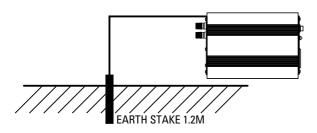
• External Earthing Mobile Applications --Connect an earth wire (Preferably solid Green or Green with Yellow stripe) from the external earth connection (Chassis GND) on the rear of the inverter to the chassis of the vehicle or ground wires in a boat.
